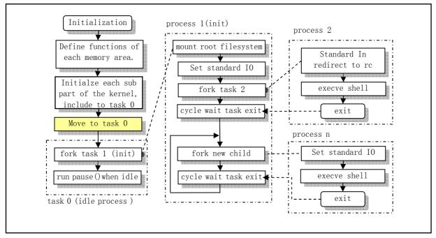
Figure 4-2 The sketch map of the procedure of kernel initialization
