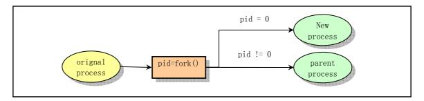
Figure 4-3 Creating new process by invoking fork()
